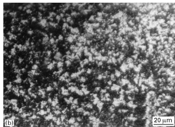
Figure 5 Microstructure of the spray deposit produced at 1.0 MPa gas pressure with a nozzle-substrate distance of 0.3 M showing (a) uniform dispersion of second phase particles and (b) high magnification micrograph of the same region.
